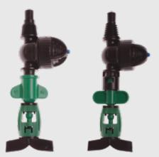
The DAN Bridgeless, the reliable predecessor of the DAN Bridgeless S, was specially developed to meet the high demands of Dutch greenhouse horticulture. It is the ideal solution when there is limited free space above the sprinkler. The Bridgeless sprinkler is installed upside down and is also available as a Cold Greenhouse (KK) version. The recommended free space above the sprinkler is 35-45 cm..
